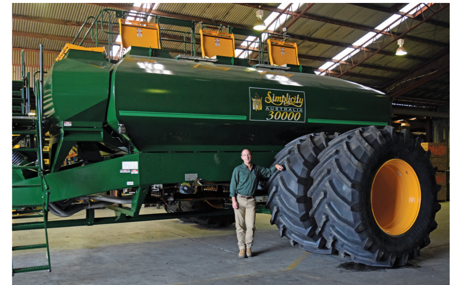
Big capacities: The 30 Series Simplicity air seeder can be up to 30,000 litres capacity.
