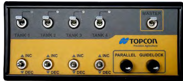
4 channel switchbox (A1267)
