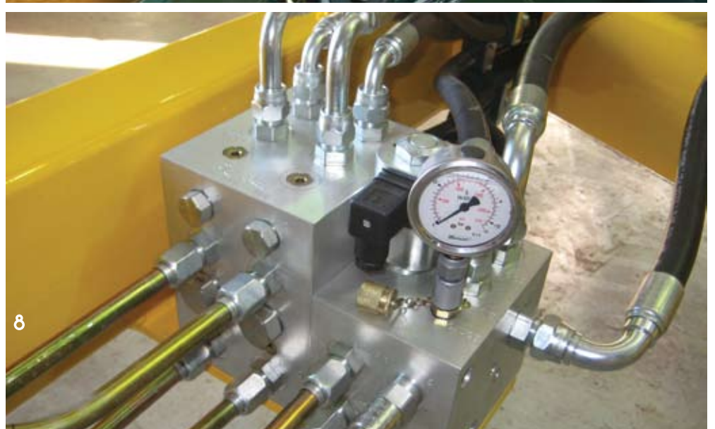
1) Dual Accumulators 2) Counter Balance Valve 3) Tyne Manifold 4) Staff Clamps 5) Hydraulic Jack 6) Visual Depth Gauge 7) Tyne Attachment 8) Hydraulic Control Block - with filter
